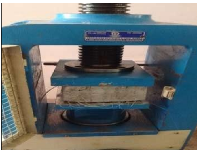
Fig 8: Compressive test of light emitting concrete
